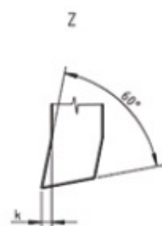
Form A: Washer with Bent Ends
